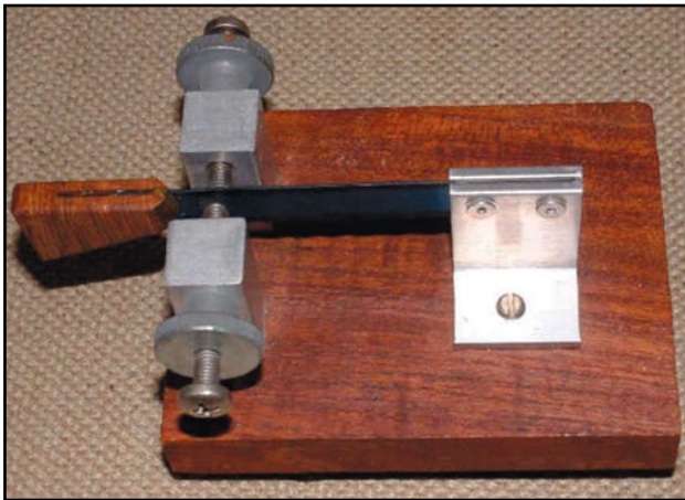
Figure 3. Sideswiper with hacksaw blade
