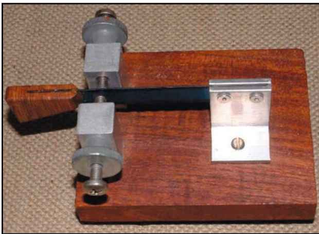
Figure 3. Sideswiper with hacksaw blade
