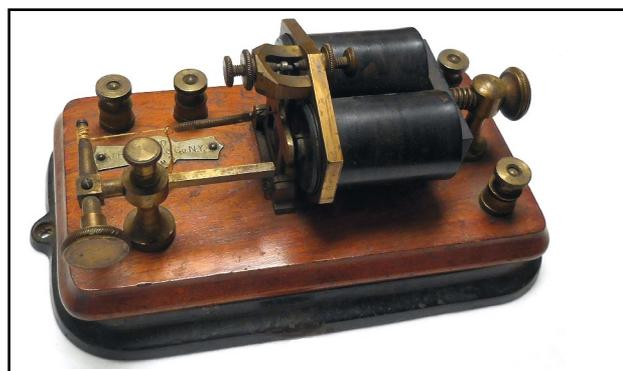
Early 1900s 150 ohm telegraph relay made by J.H. Bunnell of New York. Used to key a secondary telegraph line or sounder from a main line. From the collection of K6DF.
