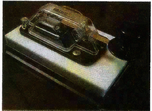
HI-MOUND, HK-808, Straight key, The touch is hard and I can send correct codes. The typing sound is loud and better use during daytime. (JL8KUS)
