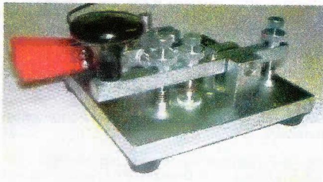
GHD, Kizuna 2012, A1CLUB key, Dual lever paddle & Straight key, I use the Kizuna with my left hand. (JA4MRL)
