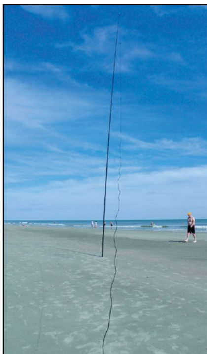
Figure 2. Jackite pole (31 ft.) strapped to 4 ft rebar rod driven 2 ft into the hard sand.
