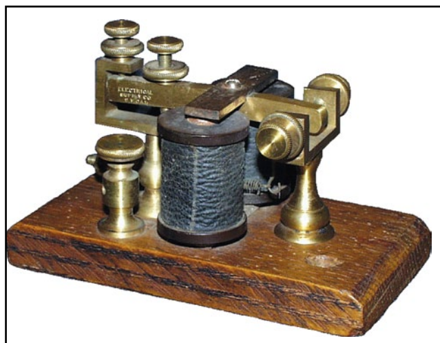
Electrical Supply Co., Telegraph Sounder circa 1848 to 1881 used on a branch telegraph line and was usually keyed by a main line relay. From the collection of K6DF.
