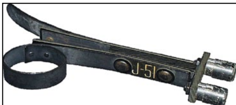
J-51 key was used a long cord to key the SE-11 Signal Lamp so the operator could get away from the lamp. Enemy soldiers would shoot at signal lamps hoping to hit the lamp or the operator. From the collection of K6DF.
