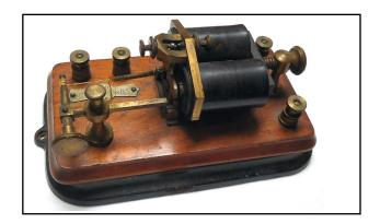
Early 1900s 150 ohm telegraph relay made by J.H. Bunnell of New York. Used to key a secondary telegraph line or sounder from a main line. From the collection of K6DF.
