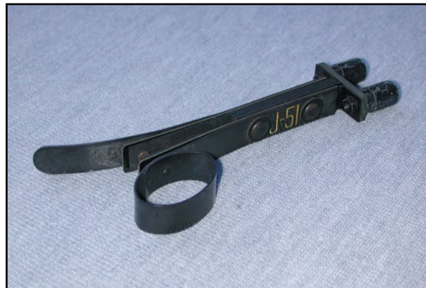
The J-51 is a very unusual key. It was used to key the SE-11 signal lamp. A long cord connected this key with the signal lamp so the operator could put some distance between himself and the lamp—enemy soldiers would shoot at signal lamps in hopes of hitting the lamp or the operator.
